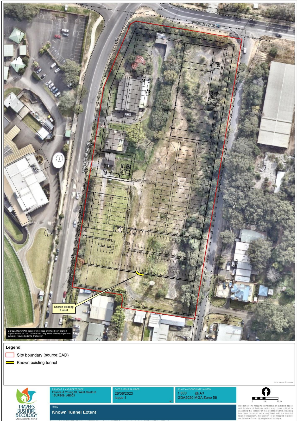
Figure 4-8: Mapped extent of subsurface tunnel within study area
